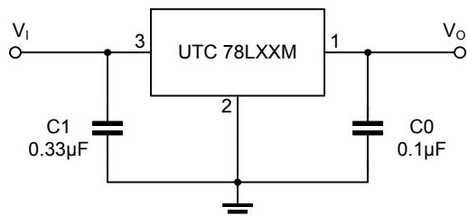
Notes 1: To specify an output voltage, substitute voltage value for "XXM".
